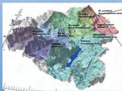
Digital elevation model with watershed, subbasins and gauges
